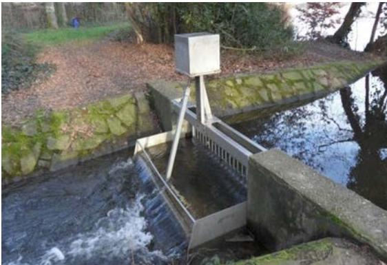
Water level measuring device, not to be mapped as construction
